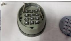
3. Remove the two black 3.0 mm hex bolts securing the keypad housing together to gain access to the circuit board.
