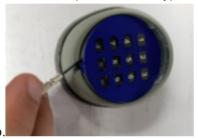
notch at the bottom center and gently pry loose with the screwdriver tip.
