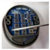
5. With access to the back of the circuit board, you will see the battery terminal and the reset (small red) button. Hold the two batteries to the battery terminal to supply power to the circuit board, while pressing the reset button. The keypad LED will light up and sound a beep. The reset has not been completed.
