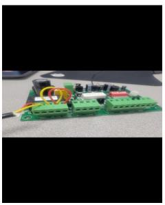
Note: This jumper test will cause the unit not to respect the magnet stop points, so ensure that you manually stop the unit before those points.
