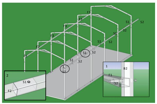
**Step 4: Assemble Roof Panels**
